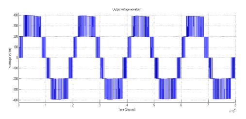
Figure (14). Output voltage waveform of five level
