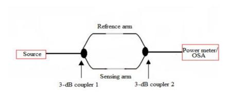
Figure (2): The schematic diagram of a MZI concentration sensor.
