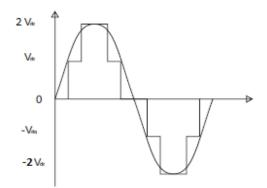
Figure (5). Output voltage waveform of five level CHBMLI [14]
