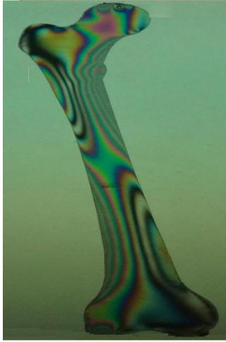
Fig.(4) Fringes pattern on femur bone under load
