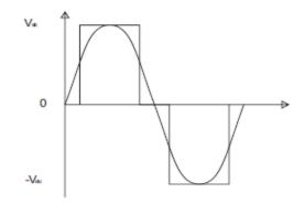
Figure (3). Output voltage waveform of three level CHBMLI [14]
