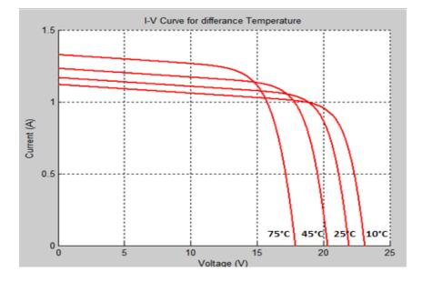
Figure 12: I-V Curve of Polycrystalline SPM020-P Model.
