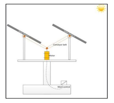
Figure 3: Proposed Design of Dual Solar Panel.
