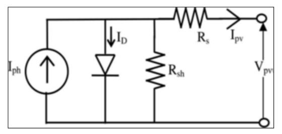
Figure 1: Equivalent Circuit of Solar Cell [3].
