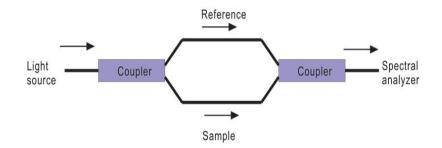
Figure (1): The schematic diagram of Mach-Zehnder Interferometer [13].
