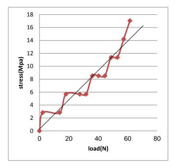
Fig. 7 Stresses with load on femur shaft
