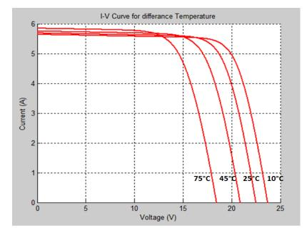
Figure 10: I-V Curve of Monocrystalline SPM100-M Model
