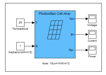
Figure 5: Simulation of Ideal Photovoltaic cell Array.
