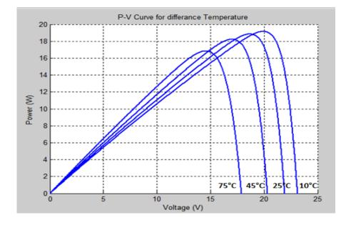
Figure 13: P-V Curve of Polycrystalline SPM020-P Model
