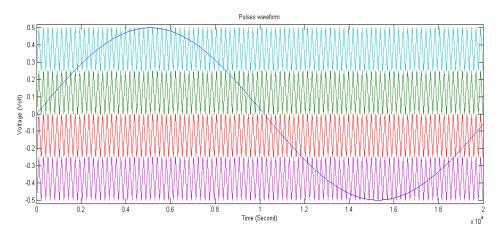
Figure (9). Carrier and Reference signals of five level CHBMLI
