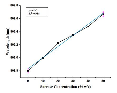
Figure (8): The relationship between wavelength and different concentrations of Sucrose solutions.
