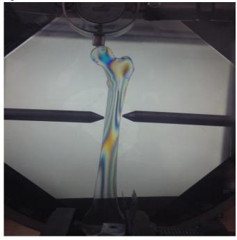
Fig.(3) Prototype of femur bone with applied load
