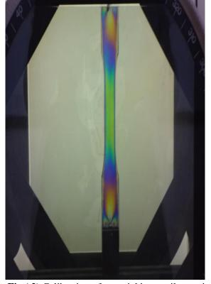
Fig.(2) Calibration of material by tensile specimen
