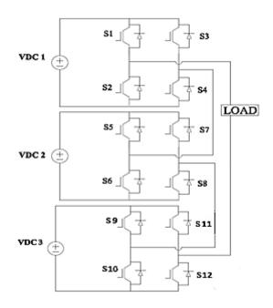
Figure (6). Circuit of seven level CHBMLI [14]
