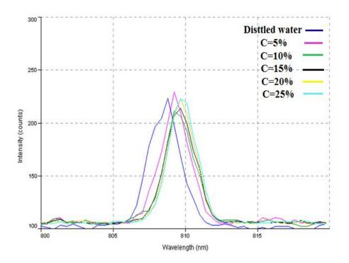
Figure (7): Interference spectra of MZI sensor for different concentrations of Nacl solutions.
