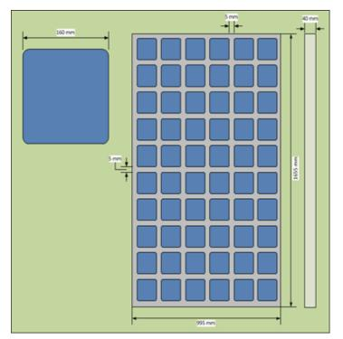
Figure 4: Dimension of Solar Panel Design
