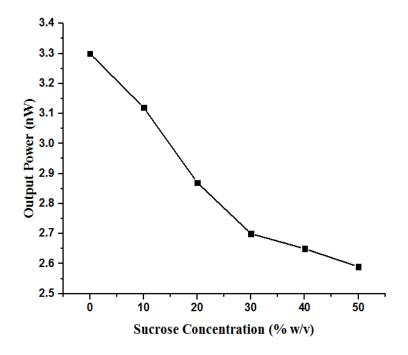
Figure (10): The relationship between output power and different concentrations of sucrose solutions.
