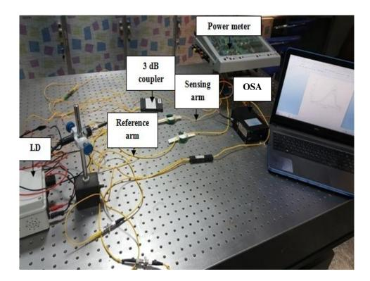
Figure (3): The experimental setup of the MZI concentration sensor.
