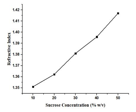
Figure (5): The relationship between concentration and refractive index of sucrose solutions.
