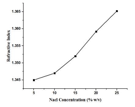
Figure (4): The relationship between concentration and refractive index of Nacl solutions.
