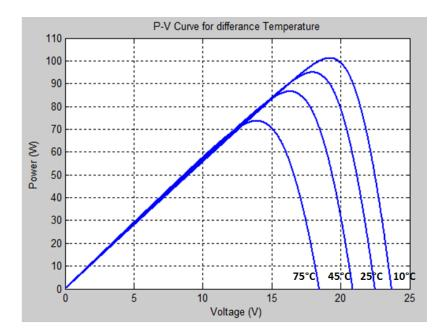
Figure 11: P-V Curve of Monocrystalline SPM100-M Model.
