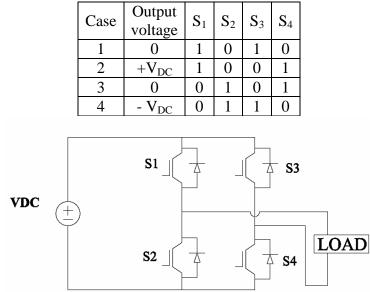
Figure (2). Circuit of single phase three level CHBMLI [14]
