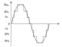
Figure (7). Output voltage waveform of seven level CHBMLI [14]
