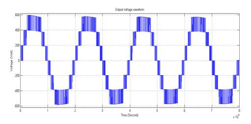
Figure (17). Output voltage waveform of seven level
