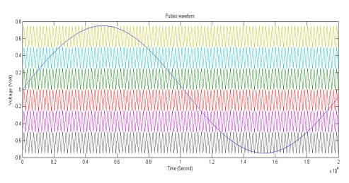
Figure (10). Carrier and Reference signals of seven level CHBMLI
